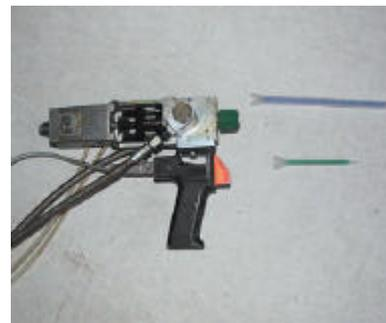
**Graphic 5 : Mobile mixing head with static mixing tube.**
